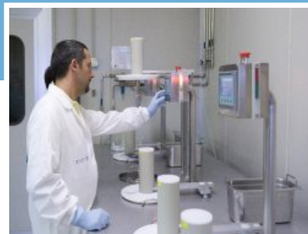
Fig. 3 – A step in the application of the Zymo-Teck process: programming the bioreactors where enzyme reactions take place.
